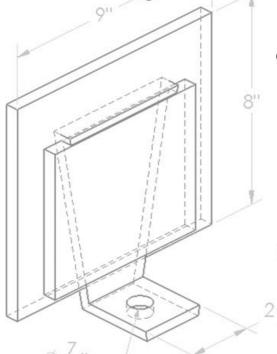
The PolyPlast Restraint System is designed primarily for cylindrical, vertical flat bottomed tanks up to 4000 gallons
