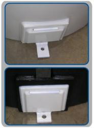
PolyPlast Restraint Systems have seismically compliant hold down lugs attached and spaced evenly around the lower tank wall. Designed with welded polyethylene plates, the PolyPlast Restraint System can be added to any of our polyethylene tanks. This system comes installed on the tank, all you have to do is bolt the tank down.
